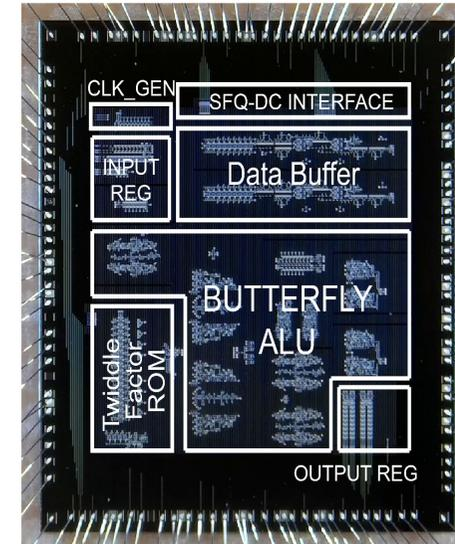
47 GHz SFQ FFT Processor [Ke et al.,2021]
