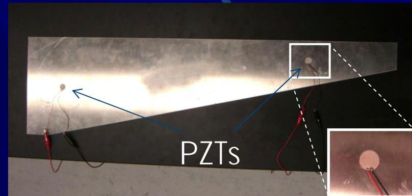
A pair of PZTs: actuator & sensor
