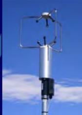
3d ultrasonic anemometer
