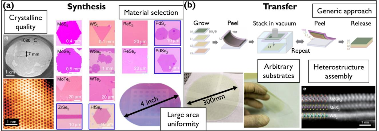
Fig. 1. Relevant metrics for synthesis and transfer of 2D materials, with notable examples. Crystalline quality and wide material selection are important to allow high performance devices. Transfer is a generic approach to allow integration in arbitrary substrates or assembly of heterostructures. Large area uniformity is essential to both synthesis and transfer, to allow low variability in material properties over wafer scales. Adapted with permission from [15]–[20].
