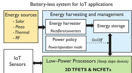
Fig. 4. Overview of Self-sustainable energy harvesting system using low power device alternatives. Adapted with permission from [129]
