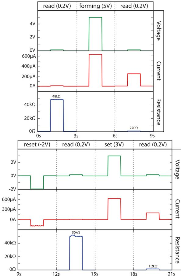
Fig. 7. Measured values of a *read-forming-read-reset-read-set-read* sequence on a memory cell, using the active current limiting circuit during *forming* and *set* operations. The device is selected using DEMUX 1 / OUTPUT 12. Naming conventions for MUXs and their connections can be found in the attached documentation [8].
