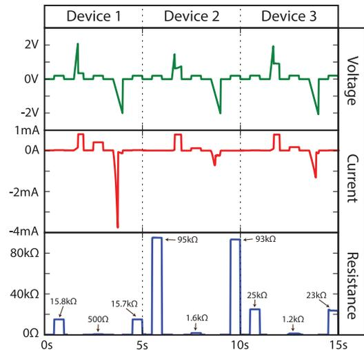
Fig. 5. Extracted portion of the time characterization sequences of three adjacent RRAM cells (Dev1 - DEMUX 1 / OUTPUT 9, Dev2 - DEMUX 2 / OUTPUT 14, Dev3 - DEMUX 5 / OUTPUT 4; naming conventions for MUXs and their connections can be found in the attached documentation [8]).
