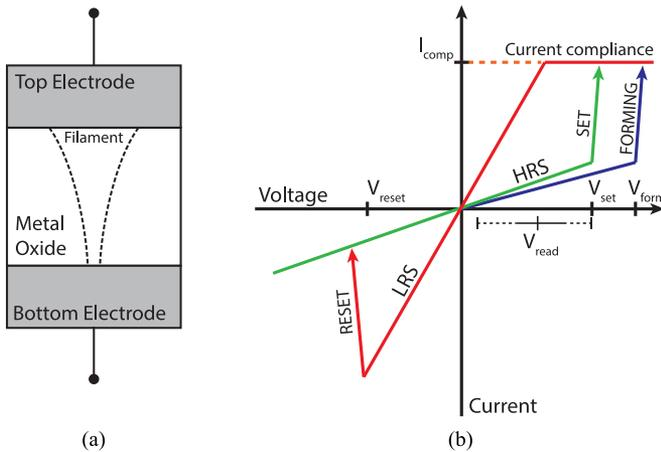
Fig. 2. (a) RRAM layer stack. (b) I-V plot of the switching mechanism.
