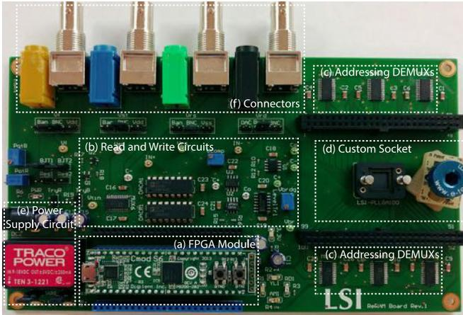
Fig. 1. Memory Characterization System (MCS) board including (a) an FPGA module, (b) read and write circuits, (c) addressing demultiplexers, (d) custom socket for the memory chip, (e) power supply circuit and (f) connectors for external equipments.
