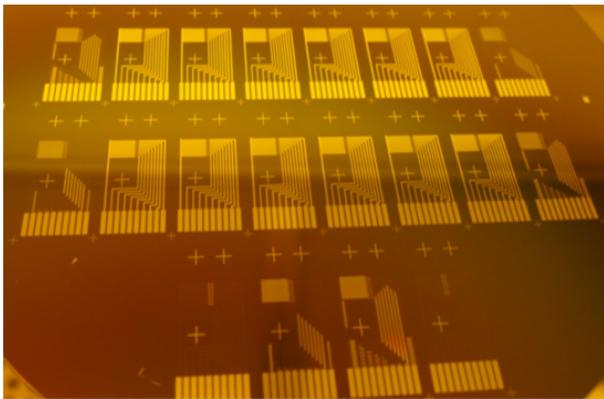
Fig. 1. SOI wafer including different configuration chips with different Al metal lines in series for assuring electrical contacts to memristive nanowire devices.
