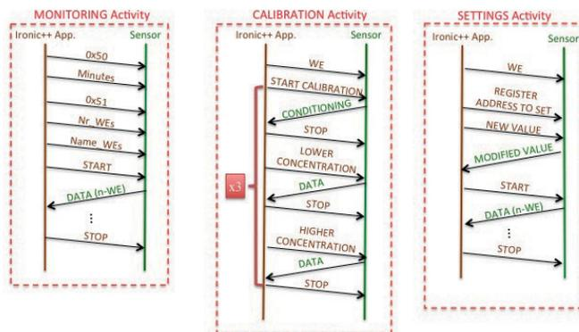
Fig. 3. Communication protocol adopted between the sensor and the Android mobile device.
