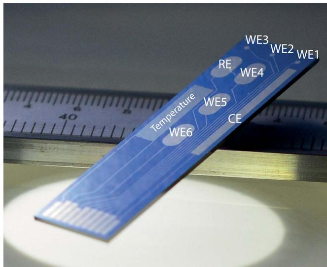
Fig. 2. *ironIC++* sensing device with six WEs, one RE, one CE and one temperature sensor.
