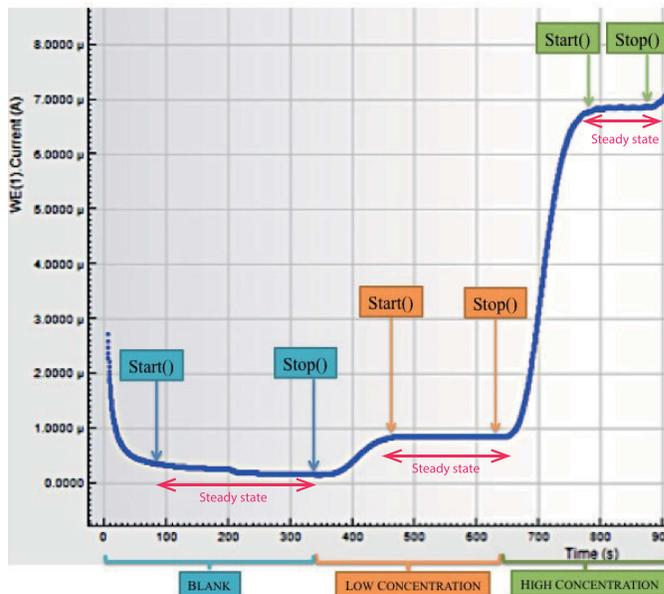
Fig. 5. Sequence of Start and Stop command send by the interface during one cycle of the calibration process.
