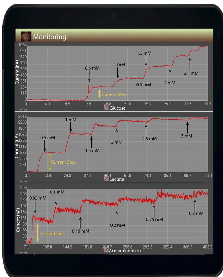
Fig. 7. Chronoamperometric results on tablet screen: measurements for endogenous glucose and lactate and exogenous acetaminophen. The SNR is evaluated in Matlab\_R2013a by applying a LPF on the measured signal and considering: low frequencies as signal and high frequencies as noise. This is a reasonable approximation since electrochemical reactions normally takes few ms. The obtained SNR values are: 96 dB, 93 dB, 116 dB, respectively, for glucose, lactate and paracetamol.
