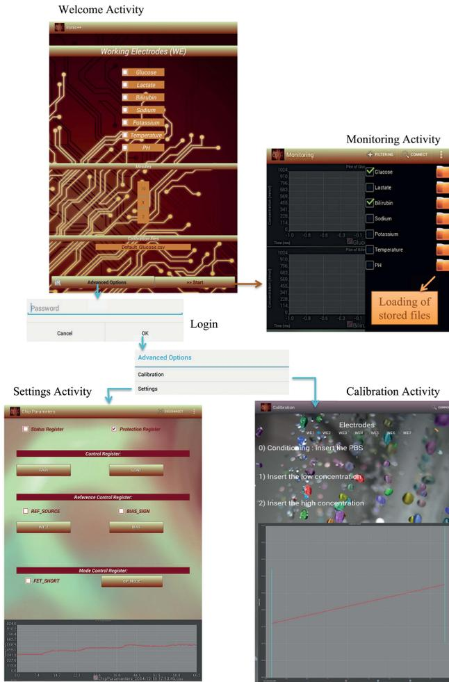
Fig. 6. Scheme with the structure of the developed Android application.
