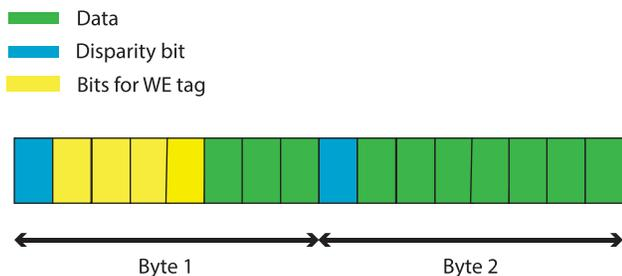
Fig. 4. Packet format for Data message.
