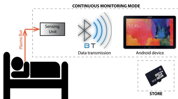
Fig. 1. Monitoring scenario where the main parameters of the patient are continuously displayed on an Android mobile device and stored in the external memory mounted on the device.
