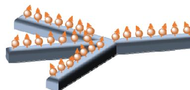
Figure 2: Sketch of a spin wave majority gate with 3 inputs and one output. The waves propagating in the 3 input arms interfere in the central region to perform the computation.
