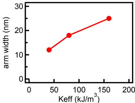
Fig. 5: STMG. Device arm width vs. effective anisotropy. Above this arm width, the failure mechanism where the domain wall becomes stuck is dominant. For  $K_{eff}$  in agreement with standard MRAM stacks, the arm width has to be lower than ~15-25nm for proper device function. Different device geometry could increase device CDs.
