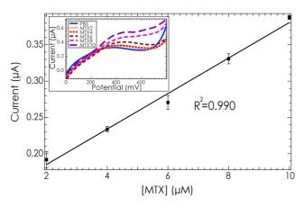
Fig. 10. Calibration curve for MTX within the physiological range in PBS, obtained in CV. Error bars correspond to the standard deviation for 4 different measurements (confidence interval 95.4%). The inset shows the oxidation peak currents increasing with the drug concentration.
