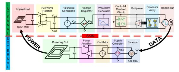
Fig. 2. Block diagram of the implantable biosensor system.
