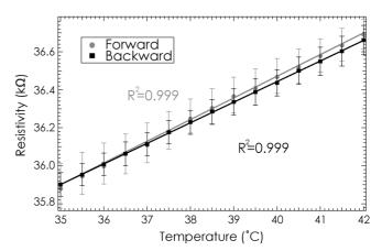
Fig. 11. Calibration curve for the temperature sensor (forward and backward scans), for a temperature range between  $35^{\circ}$ C and  $42^{\circ}$ C.
