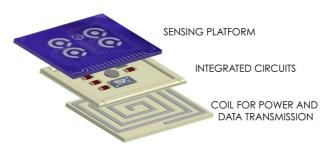
Fig. 7. Scheme of the integrated device assembly.
