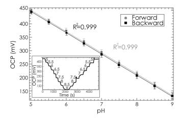
Fig. 12. Open circuit potential of the IrOx coated electrode to different pH. The inset shows the OCP measurements versus time. The OCP steps correspond to different pH levels.
