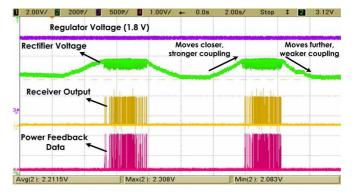
Fig. 4. Remote powering signals and power feedback data for power adaptation.
