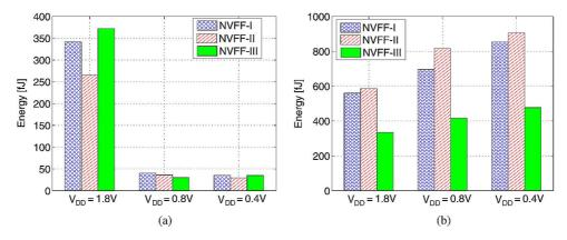
Fig. 6. (a) Read energy; and (b) write energy comparisons for different main supply voltages V<sub>DD</sub>. Note that the voltage is always risen to 2.4 V for ReRAM write.
