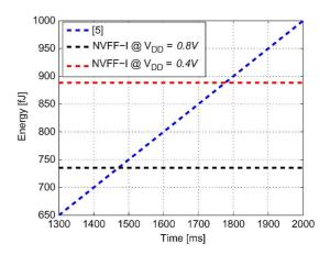
Fig. 7. Energy break-even sleep time of NVFF-I w.r.t. low-leakage CMOS latch [23].
