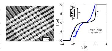
Fig. 1.  $1.5 \ \mu m^2 \ Al/TiO_2/Al \ ReRAM$  stack crossbar SEM image and single node switching characteristic under 10  $\mu A$  current compliance. The crossbar structure is solely used for device characterization, while all NVFF topologies contain only one or two separate ReRAM stacks.
