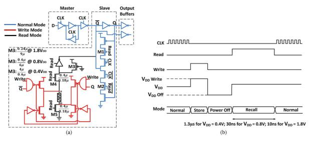
Fig. 4. (a) NVFF architecture with a single ReRAM device (NVFF-III); and (b) the corresponding control sequence for read and write operation.
