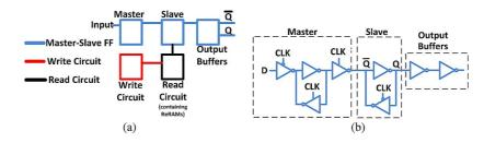
Fig. 2. (a) Conceptual block diagram of a non-volatile flip-flop; and (b) conventional master-slave flip-flop.
