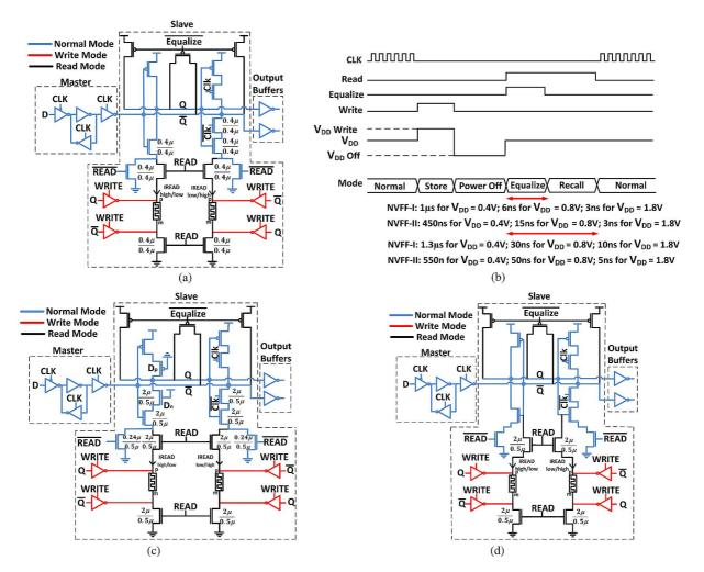
Fig. 3. (a) Baseline non-volatile flip-flop design (NVFF-0); (b) control signals sequence for ReRAM read and write operations for the complementary ReRAMbased NVFF circuits; (c) sub- $V_{\rm T}$  optimized NVFF structure, based on NVFF-0 topology (NVFF-I); and (d) sub- $V_{\rm T}$  optimized NVFF structure, inspired from [18] (NVFF-II).
