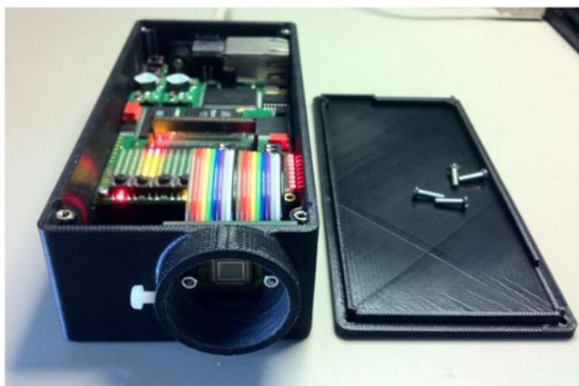
**Fig. 2** Custom-designed CMOS camera
