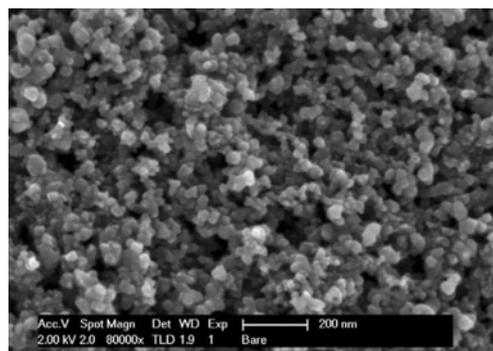
**Fig. 3** SEM image of a bare screen-printed electrode
