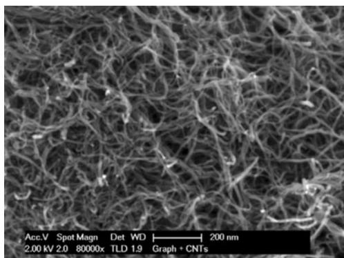
**Fig. 2** SEM image of multiwalled carbon nanotubes onto a screen-printed electrode
