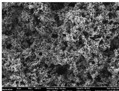
**Fig. 1** SEM image of silicon carbide nanoparticles onto screen-printed electrodes
