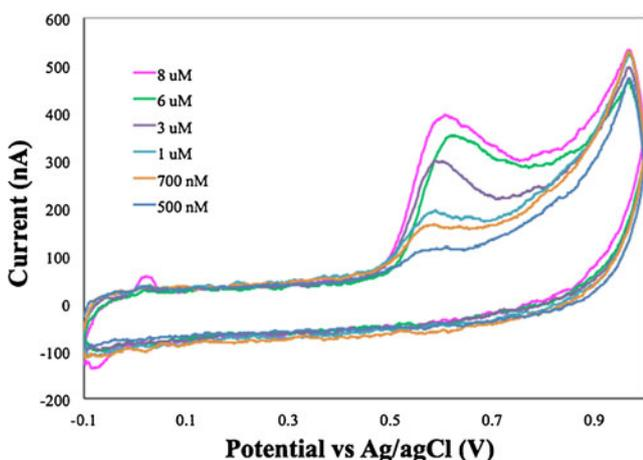
**Fig. 4** Cyclic voltammograms on insulin at different concentrations as gathered on a bare screen-printed electrode
