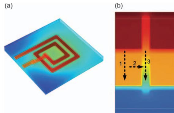
**Fig. 7.** Temperature variation (a) across an inductive link and (b) along a TSV.
