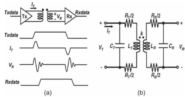
**Fig. 2.** Basic operation of an inductor link, where (a) is the inductively coupled transceiver and (b) is the equivalent circuit for the spiral inductor.<sup>27,28</sup>
