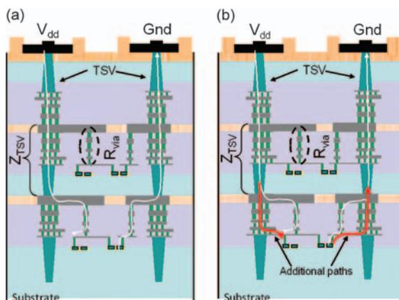
**Fig. 5.** Current paths within a 3-D circuit, (a) where the TSV is connected only to the topmost metal layer and (b) where the TSV is connected to the power lines on both the uppermost (MT) and the first (M1) metal layers of a circuit plane. TSVs are formed with a “via-middle” process.
