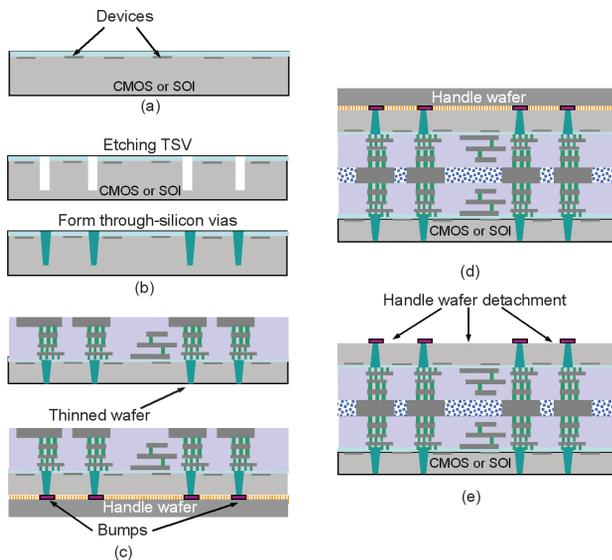
**Fig. 1.** Basic steps of TSV manufacturing for a “via-middle” process, (a) wafer preparation and FEOL, (b) TSV etching and metal filling, (c) wafer thinning and BEOL, (d) wafer bonding, and (e) handle wafer removal.
