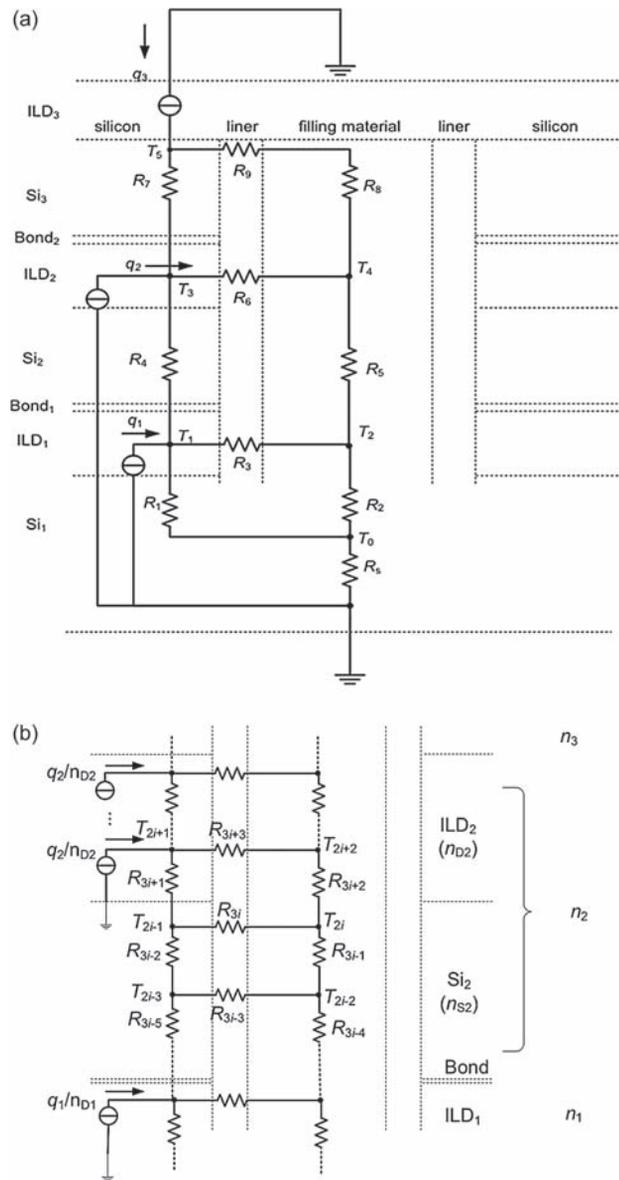
Fig. 6. Thermal model of a TTSV in a three-plane circuit where (a) is the compact model and (b) is the distributed model.
