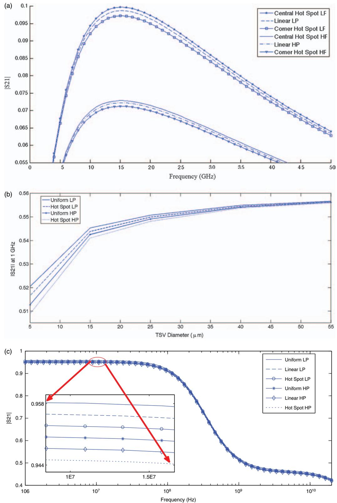
**Fig. 8.** Amplitude of  $|S_{21}|$  for three temperature profiles (a) for an inductive link and (b) for TSV stack with different diameters at frequency of 1GHz, and (c) for TSV stack with diameter of  $5 \mu\text{m}$ .
