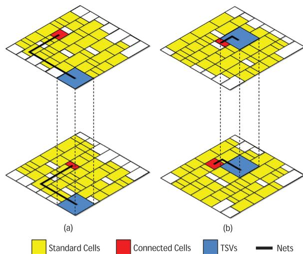
Fig. 4. Different TSV allocations for 3-D circuits where in (a) no active area for TSVs is reserved during placement and in (b) some active area for TSVs is reserved during placement.<sup>13</sup>
