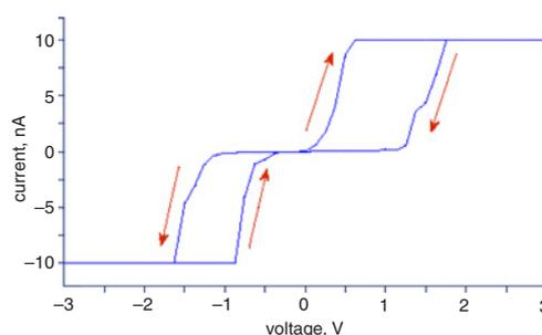
**Fig. 3** Post-forming I-V characteristics showing pinched bow-tie loop
