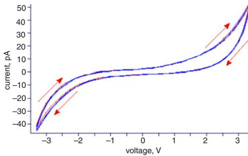
**Fig. 4** Pre-forming  $I$ - $V$  hysteresis loop comprising four sweeps
