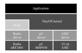
Figure 1. OS-Based EEG/ECG 24+1ch sensor node architecture overview
