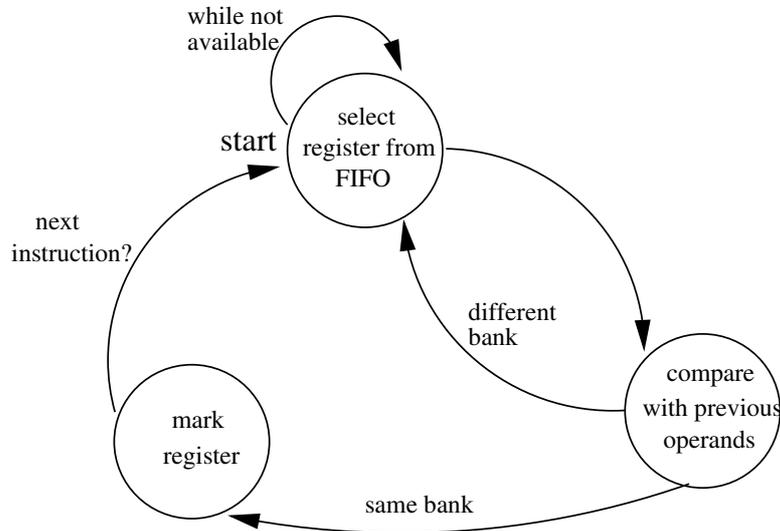
**Fig. 2.** Register assignment algorithm
