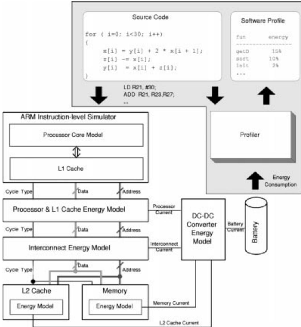
Fig. 10. Profiler architecture.
