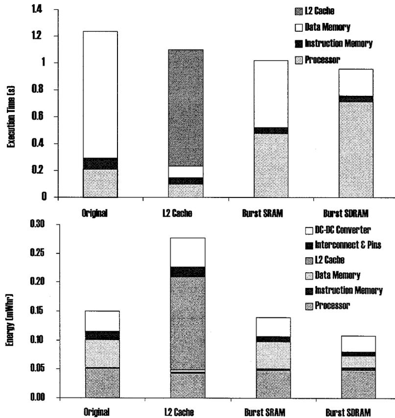
Fig. 6. Performance and energy consumption for hardware architectures.
