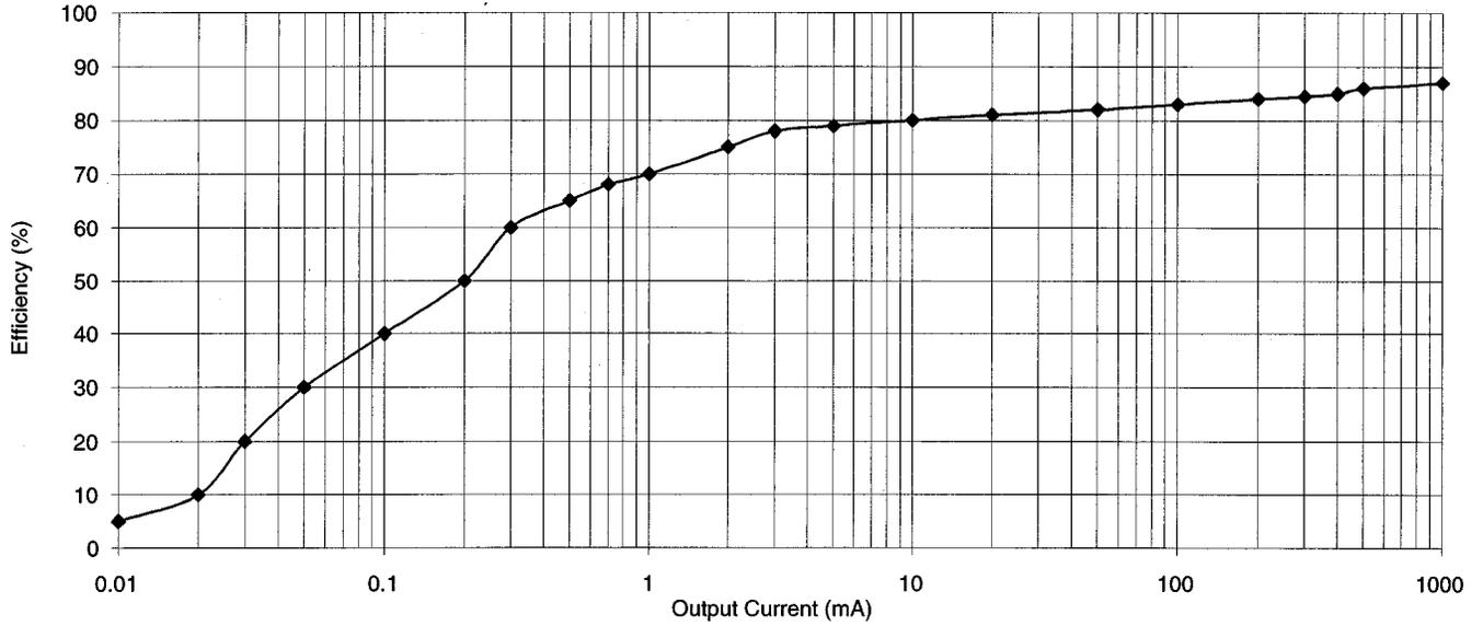
Fig. 3. DC-DC converter efficiency.
