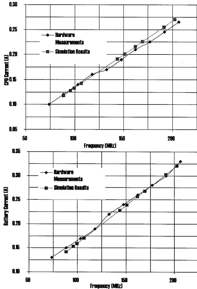
Fig. 5. Average processor core and battery currents.
