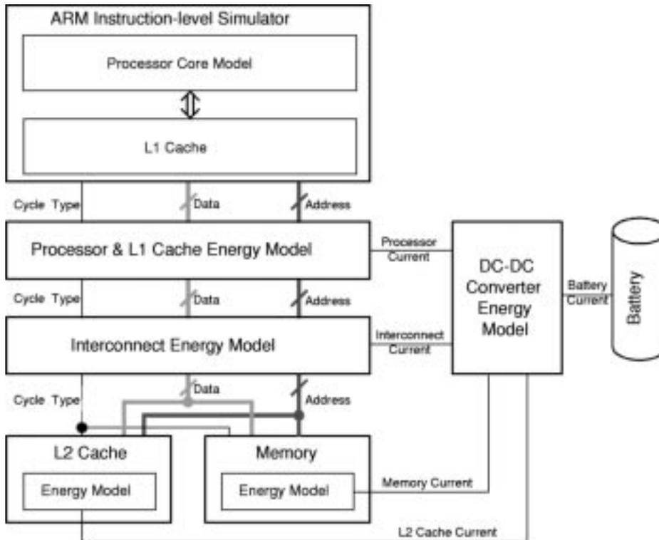
Fig. 2. Simulator architecture.
