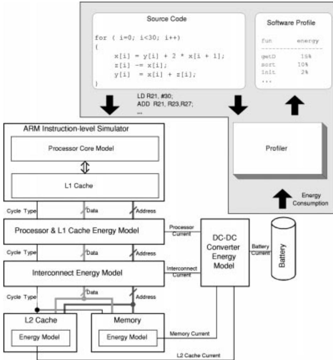
Fig. 10. Profiler architecture.
