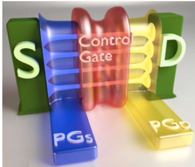
Figure 3.4: Schematic of three-independent-gate SiNWFET.
