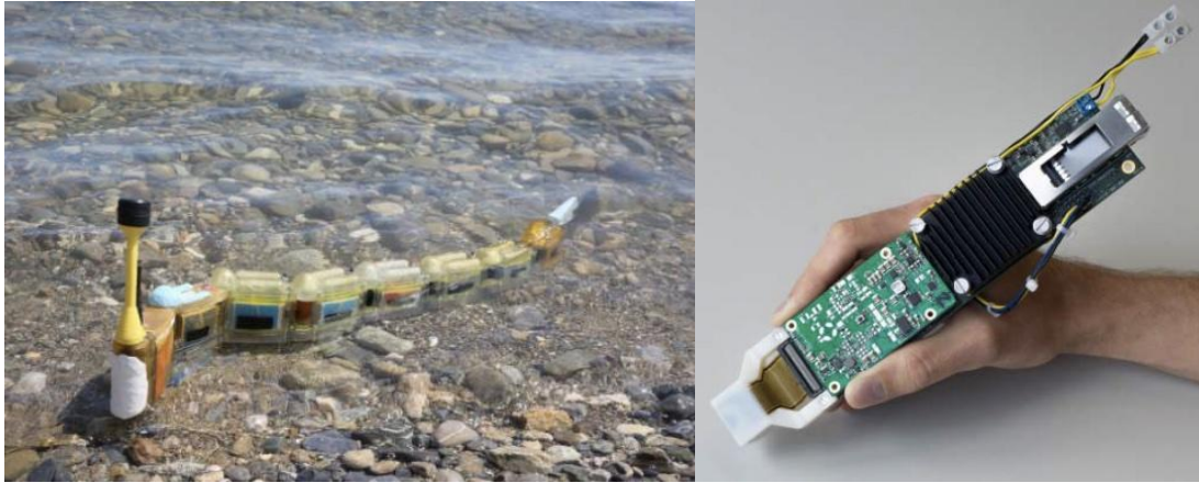
Figure 13. Some outcomes of the Nano-Tera Program. (a) Autonomous swimming robot searching for pollutants in fresh water. (b) Probe of a portable 3D ultrasound system for remote diagnosis.
