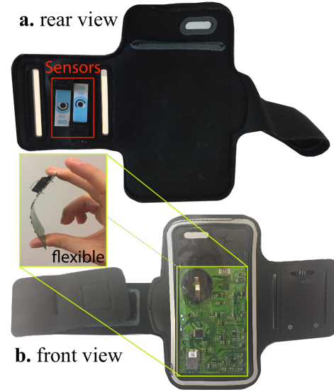
Fig. 6: Integration of the electrochemical platform in an armband: a. rear view b. front view.
