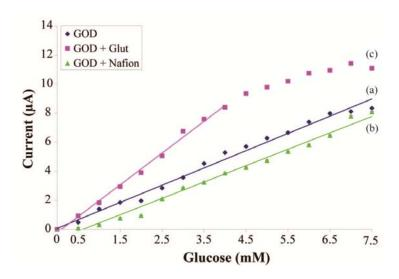
**Fig. 2.** Wider linear range: (a) adsorbed GOD; (b) GOD entrapped in Nafion; and (c) GOD cross-linked with glutaraldehyde. Data are represented as means  $\pm$  SD.
