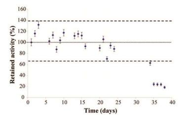
Fig. 5. Stability of the entrapped GOD in a Nafion matrix for the detection of 2.5 mM glucose. The applied potential was +550 mV. Data are represented as means  $\pm$  SD.
