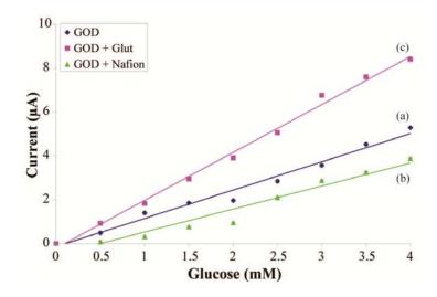
**Fig. 1.** Linear range: (a) adsorbed GOD; (b) GOD entrapped in Nafion; and (c) GOD cross-linked with glutaraldehyde. Data are represented as means ± Standard Deviation (SD).
