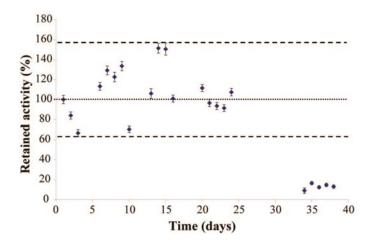
**Fig. 4.** Stability of the adsorbed GOD onto the electrode surface for the detection of 2.5 mM glucose. The applied potential was +550 mV. Data are represented as means  $\pm$  SD.
