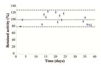
**Fig. 6.** Stability of the cross-linked GOD with glutaraldehyde for the detection of 2.5 mM glucose. The applied potential was +550 mV. Data are represented as means  $\pm$  SD.
