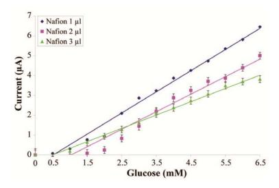
**Fig. 3.** Calibration line for GOD entrapped in different quantities of Nafion. Data are represented as means  $\pm$  SD.
