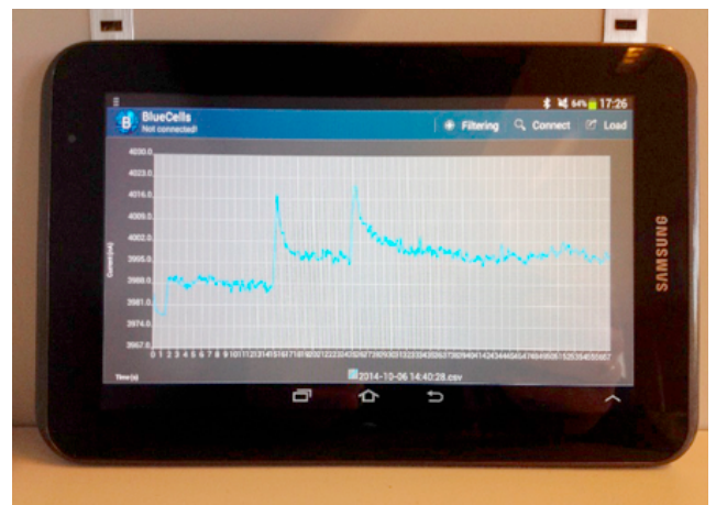
Fig. 7. Chronoamperometry on the Android interface
