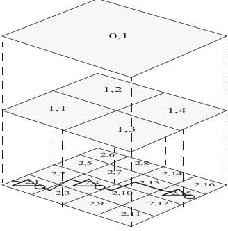
Fig. 1. Modeling spatial correlations using quad-tree partitioning [12].
