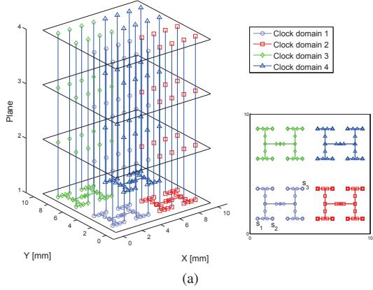
Fig. 3. Different assignments of clock domains in a four-plane 3-D IC. (a) Four clock domains within each plane. (b) Two clock domains within each plane (a total of four clock domains).
