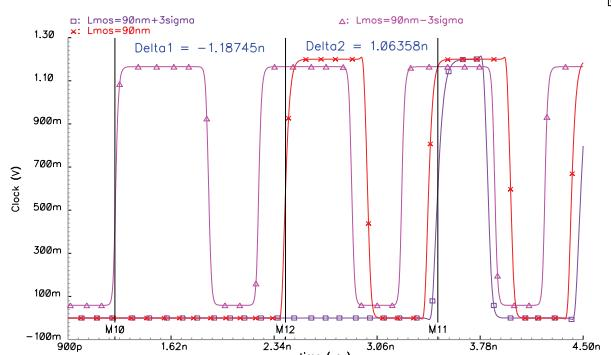
Fig. 4. Waveform of the signal at  $s_1$  with different gate lengths of MOSFET.
