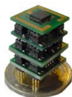
Figure 1. Sensor Cube on a 2 Euro coin
